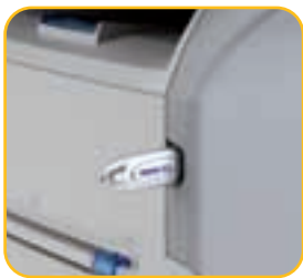
Wireless printing thanks to a WLAN dongle connected to the machine.
